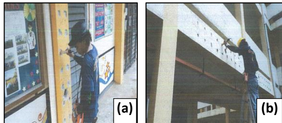
Fig. 4. The potential readings is recorded at every location on marked grid on (a) the sides of column and (b) on the sides of beam.
