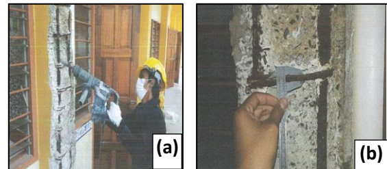
Fig. 5. Concrete column is being hacked (a) to expose reinforcement bar for measurement (b).
