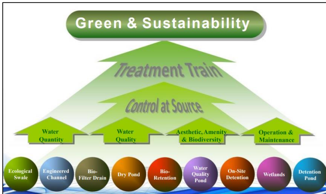
Fig. 1. The objective, principle and the components of BIOECODS
