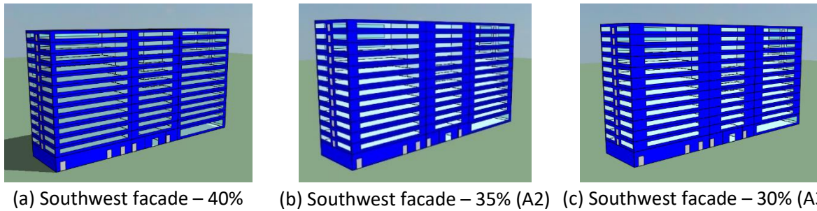
Fig. 3. The modified case models according to the proposed WWR reductions.
