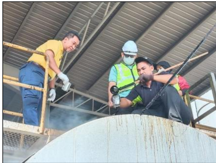
Fig. 4. WMB samples were taken from bitumen tank at quarry.
