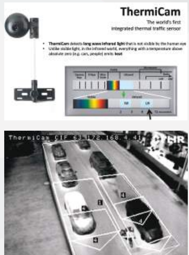
Figure 3: FLIR Thermicam, Detection Zone & Region
