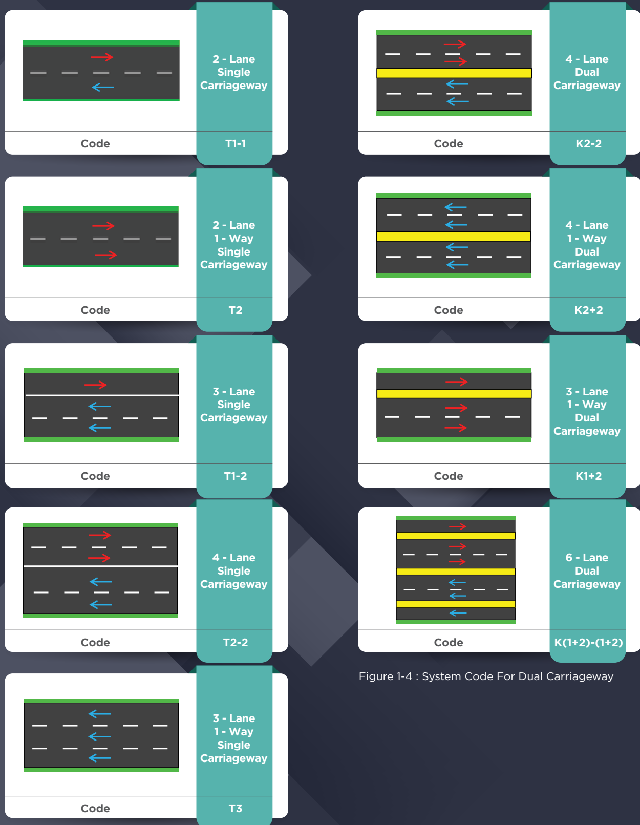
Figure 1-3 : System Code For Single Carriageway
