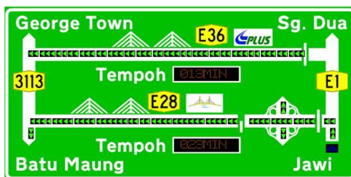
Figure 21 : Dynamic road signage on Jambatan Sultan Abdul Halim Mu'adzam Shah
