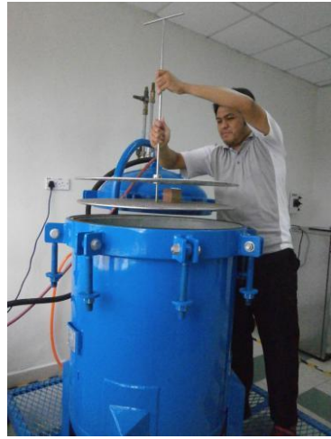
Fig. 5. Test Preparation for the delamination test
