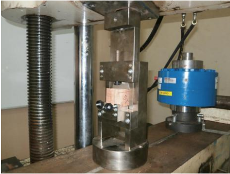
Fig. 7. Test setup for Block Shear test
