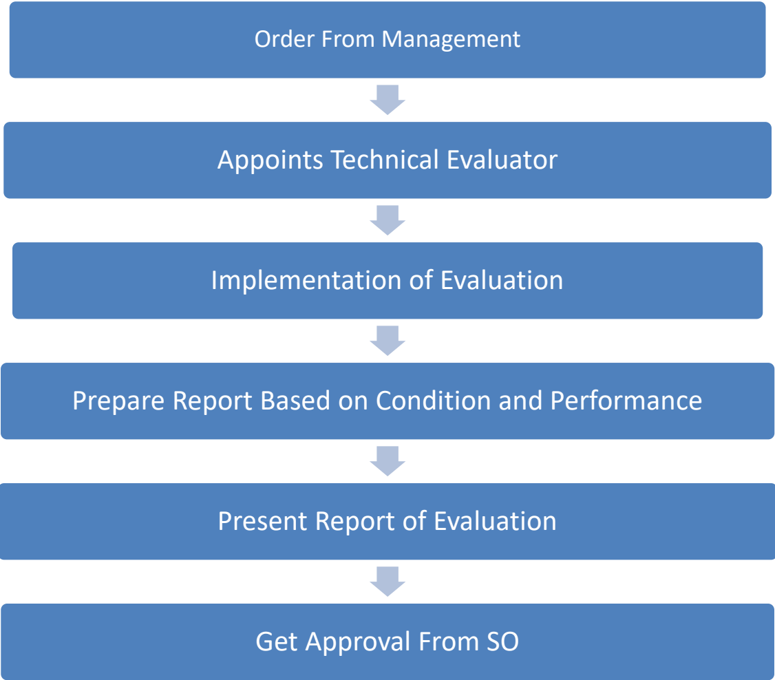
Fig. 1. JKR.PATA.F8-5: Asset Building Evaluation Procedure (Page 136: Item 5. Carta Prosedur E2, TPATA 2012, Malaysian Government)
