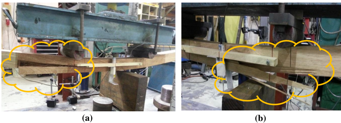
Fig. 12. (a)-(b) Failure of Glulam beam
