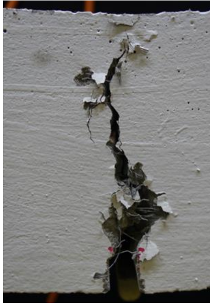
Fig. 7. Sewing effect of steel fibre in CF specimen.
