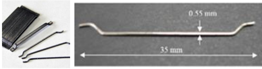
Fig. 1. Hooked end steel fibre geometries.
